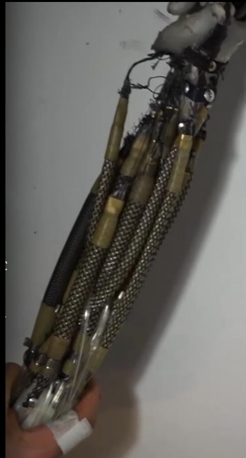
Artificial Muscles Robotic Arm, Real Copy of Human Arm, https://www.youtube.com/watch?v=gd9d_BAXWvg
