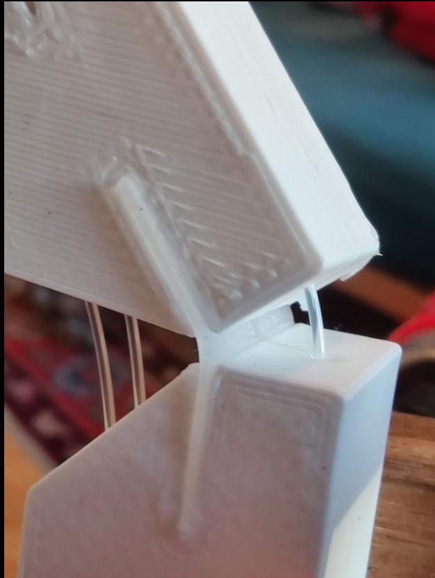
Flexure joint using polypropylene sheets
